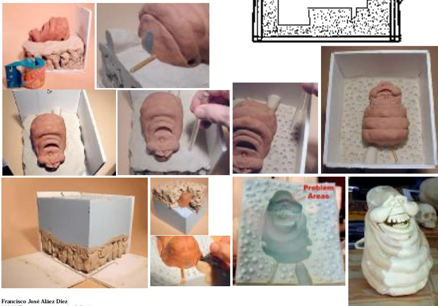
MOLDES DE RECUBRIMIENTO (GUANTE) CON SILICONA VERTIDA
